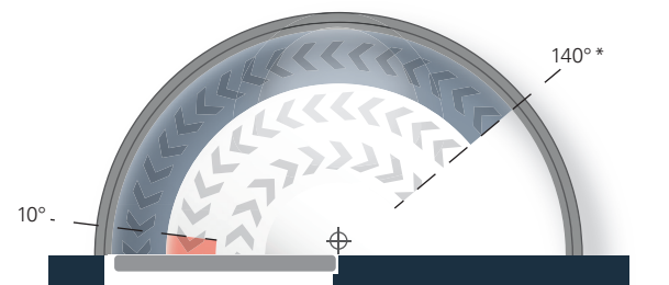
Closing force diagram Newton TS-31, hinge-opposite side
