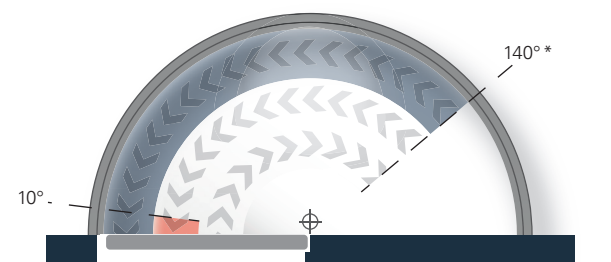
Closing force diagram Newton TS-31, hinge-opposite side
