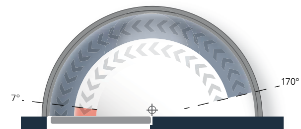
Closing force diagram ECO Newton TS-16, hinge-opposite side
